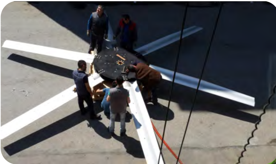
Fans for cooling towers
